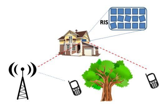
The recent research results confirm that effective deployment of RIS as controllable surfaces can enhance network capacity and coverage, but also create opportunities for future applications such as positioning and localization. The RIS can be designed as a self-configuring and part of a wireless network infrastructure, adjusting its electromagnetic characteristics in response to dynamic traffic demand and propagation characteristics.
