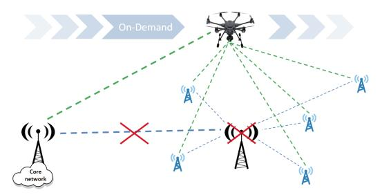
Figure 5 - Fronthauling topology (blue) replaced by alternative links (green) by using a drone
