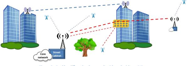
Figure 3 - Backhaul/fronthaul network with and without RIS
