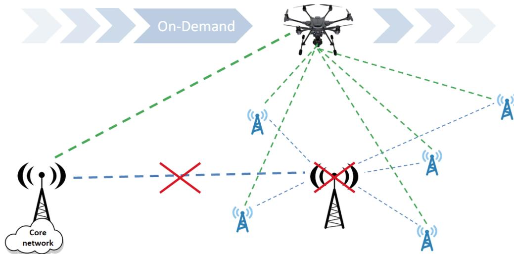
Figure 5 - Fronthauling topology (blue) replaced by alternative links (green) by using a drone
