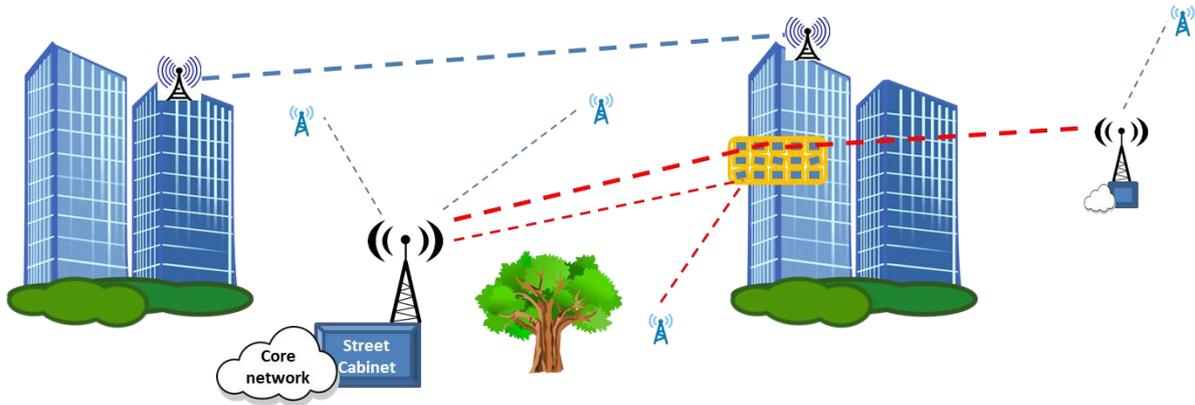
Figure 3 - Backhaul/fronthaul network with and without RIS
