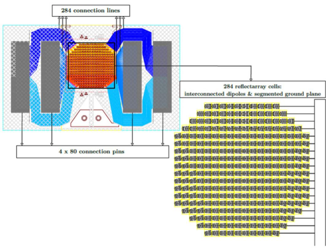
A third element of the ARIADNE toolbox are high gain and beam-steering antennas, which enable the alignment and switching to installed metasurfaces of a radio cell. A very attractive candidate to achieve the beamswitching function is application of relectarrays. ARIADNE has recently investigated the first LC-based antenna prototype with 286 array elements at W-band. The scaling of
