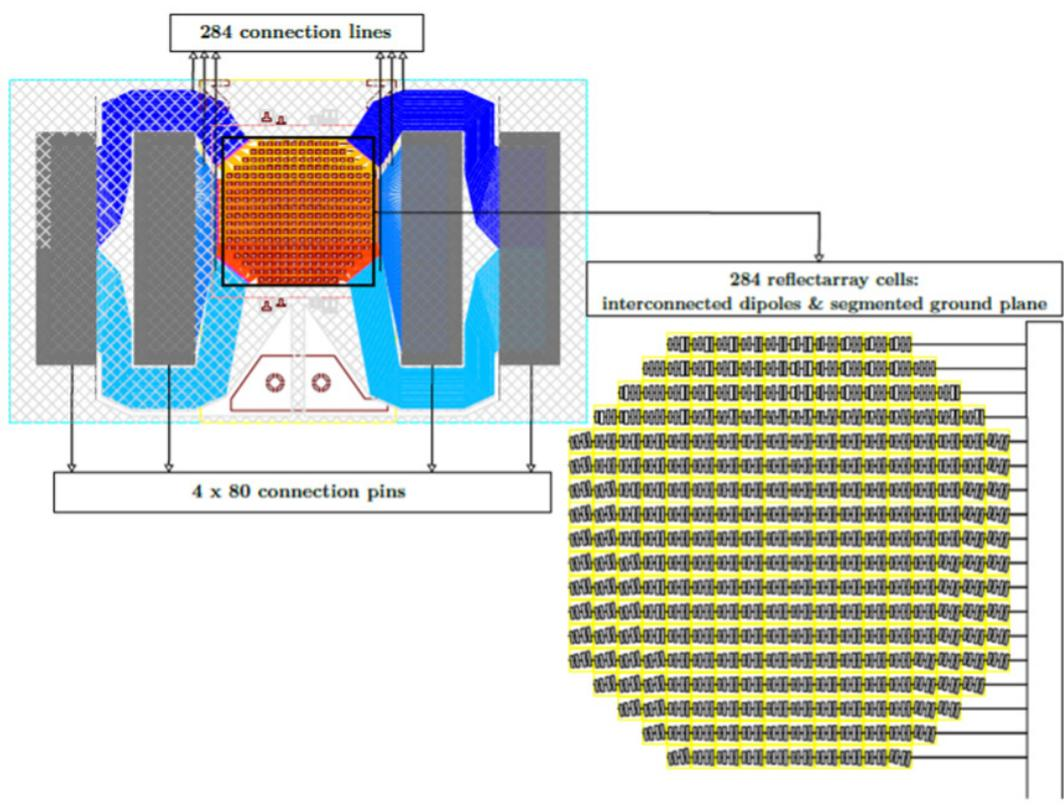
A third element of the ARIADNE toolbox are high gain and beam-steering antennas, which enable the alignment and switching to installed metasurfaces of a radio cell. A very attractive candidate to achieve the beamswitching function is application of relectarrays. ARIADNE has recently investigated the first LC-based antenna prototype with 286 array elements at W-band. The scaling of
