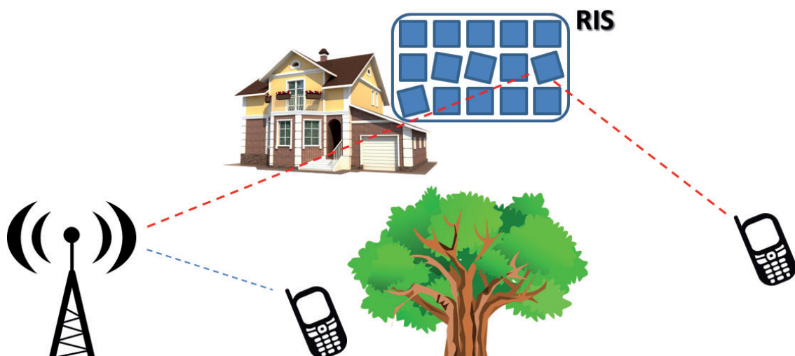
RIS attached to a house enabling communications avoiding obstacles
